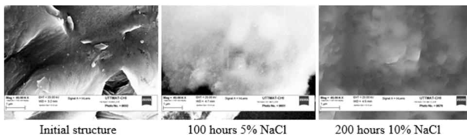
Fig. 6. Microstructural changes at 40000x magnifying scale
