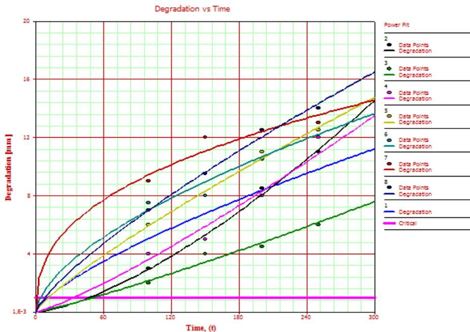
Fig. 2. The degradation obtained from the accelerated tests in accordance with the inspection time of the specimens
